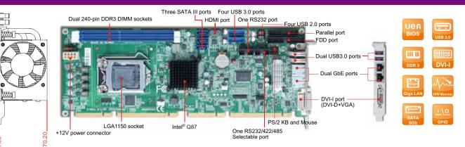
ROBO-8112VG2AR-Q87 is based on Intel Q87 chipset and workstation processor sku like Core™ i5/i7. Build with flexible PCI express expension, it's suitable for Medical, Industrial automation, and digital signage applications.
